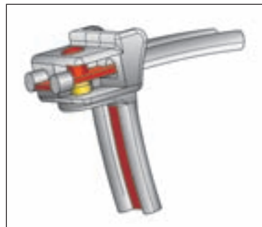
The cable tie (red) is locked into place with the pin.
